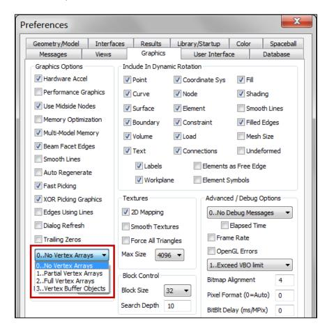
• MAX VBO should be set in a range from 50 to 75 percent (%) of the total graphics card memory of the installed graphics card.
