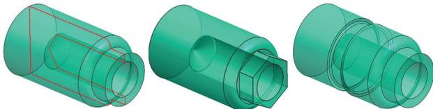
Turning > Milling > Turning
