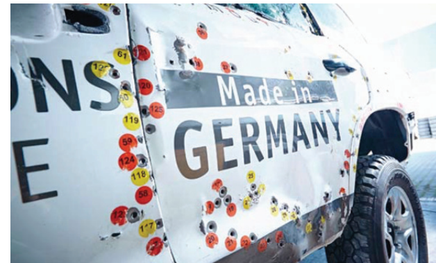
Live-fire test for certification. Copyright: Farmingtons Automotive GmbH.
