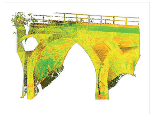
3D scan of one arch. Copyright: Ingenieurbüro Dr. Saueremann – Orlicek – Rohen GmbH.
