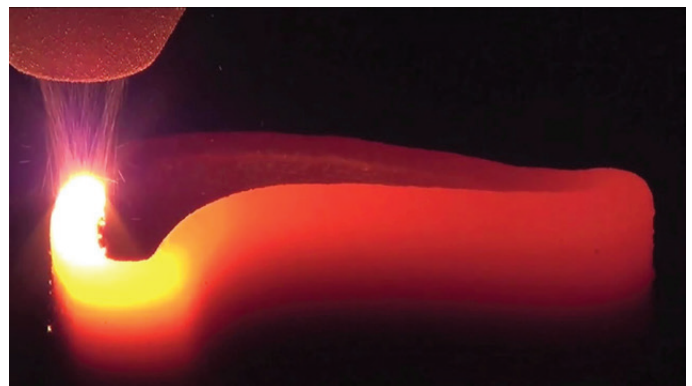
3D printing with a metal deposition nozzle.
