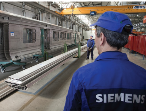
Aluminum ribs that form the car chassis on the production line.
