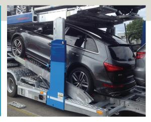
Load-bearing parts such as this loading board must be small, light and multi-adjustable, and sustain growing stresses from increasingly heavy
