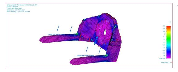
"In many cases, they are simply budgetary estimates, but with early simulation our confidence in these estimates is greatly improved. Early use of FEA speeds the process. Hand calculations for loadings on key structural members that could take hours in the past can be done in 20 to 30 minutes now."
