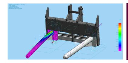
Finite element analysis results on a cantilever beam loading check. Shown is a custom-manufactured fortistic attachment that handles steel coils.
