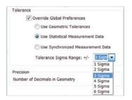
analyzing various designs or supplier components and aids in debugging a complex model. For example if a particular part is giving you erratic results, you can see how much variation goes away if the part is held to nominal values.
