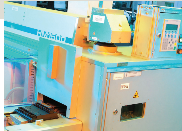
Customized laser marking of a manufactured electronic assembly.
