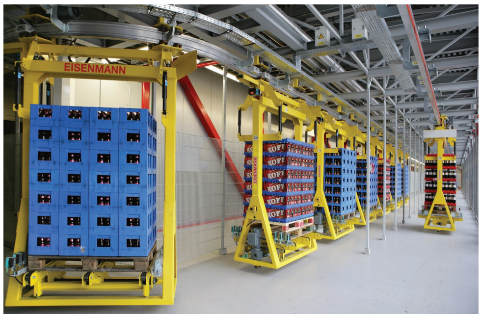
Eisenmann electrified monorail system.
