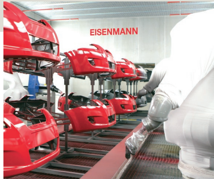
Automotive subassembly paint line delivered by Eisenmann.
