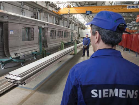
Aluminum ribs that form the car chassis on the production line.
