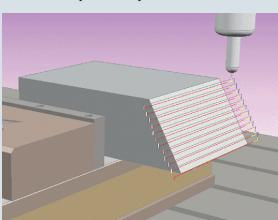
Choose an axial depth of cut of about 1/3 of the tool diameter. Use the tool supplier's recommendations to choose a chip load. Both parameters will remain constant throughout the testing. Lexmark used a 4 mm depth of cut and a chip load of 0.072 mm/tooth.
