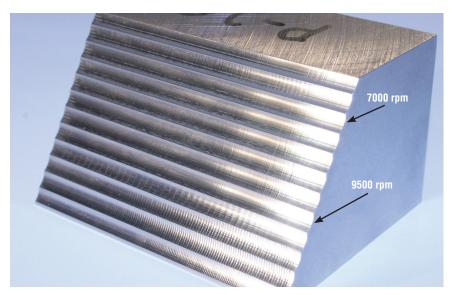
Here is a test workpiece, photographed after machining the last stepover depth listed in the chart on the facing page. Stable cutting occurred at 7,000 rpm and 9,500 rpm.
