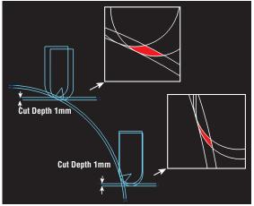
can be made an integral part of toolpath generation. By providing high speed machines with tool paths designed to keep the material removal rate consistent, a mold shop can realize the full benefits of hard milling.
