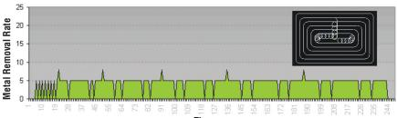
For the same depth of cut, differences in the tool's engagement can change the tool loading and the surface finish.
