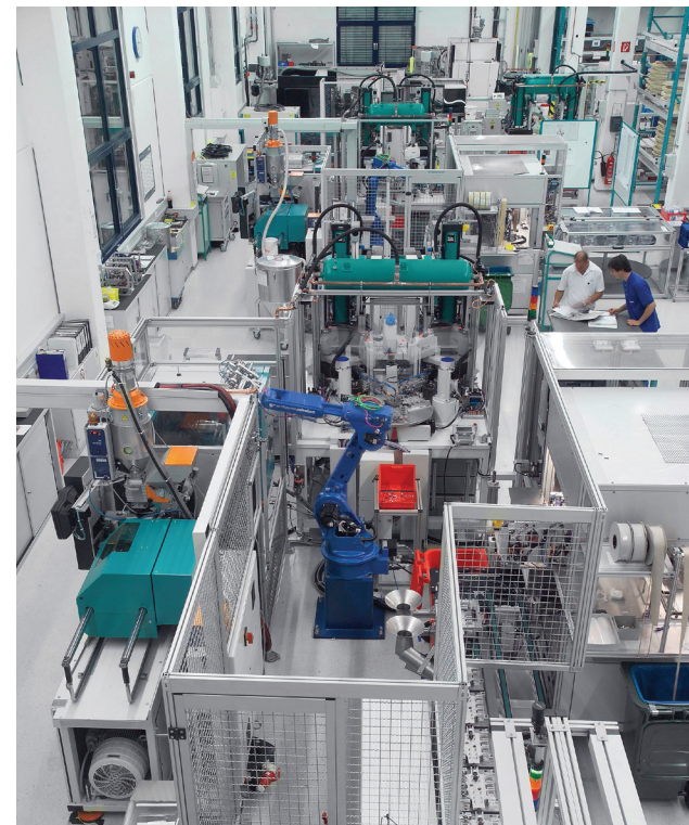
Fully automated production line that includes stamping, bending and injection molding operations.
