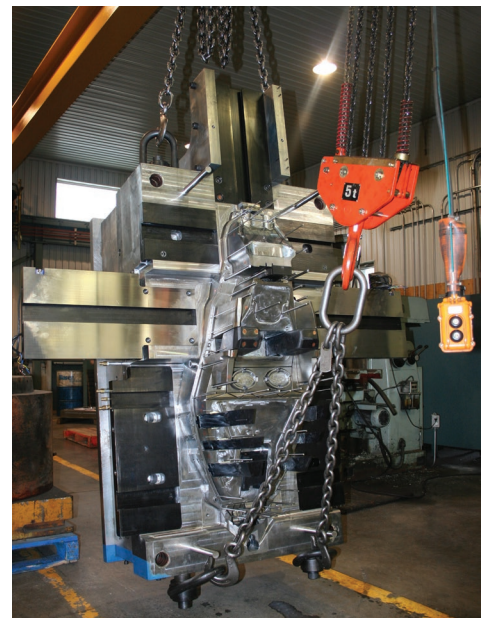
"B" side of mold – virtual and physical.
