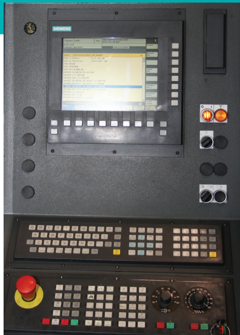
SINUMERIK 840D controller applied to mold and die machining.
