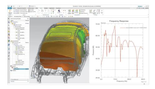
You can also use nonhomogeneous materials in the AML region to account for gradients in material properties. NX Nastran can also be used to accept the specifications of multiple AML boundary conditions.
