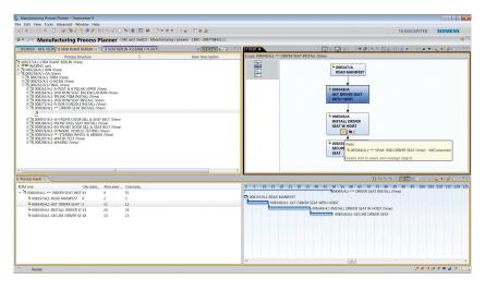
showing the dependencies and constraints while the latest enhancements to the Pert Chart capabilities further refine the synchronization between processes and the parts/assemblies tied to specific operations. Now parts, resources and manufacturing features are directly tied to the Pert Chart components which streamline the sequencing of operations and improve change management with intuitive visual cues in a single window.
