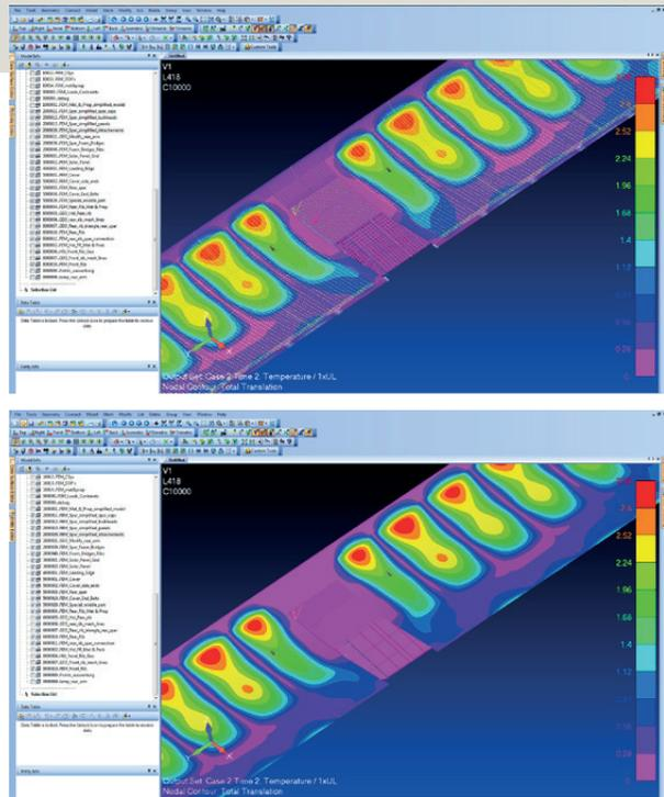
highest stresses, quickly showing where the failures are in the laminate or sandwich structure. “Scripts such as these save time and, equally importantly, help ensure the accuracy of the analyses,” says Piller.
