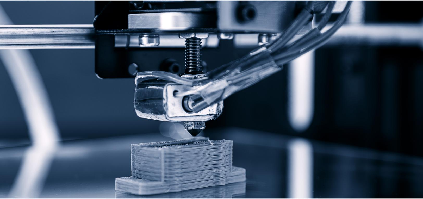
Additive manufacturing is the process of layering physical materials to create a completed product or component based on a digital twin. The most common example is 3D printing, in which printing aluminum or other materials into parts is revolutionary for component manufacturing.
