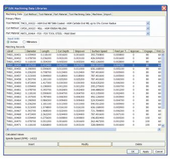
Machining parameter data is automatically drawn from the library as operations are created.
