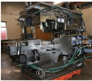
Completed mold assembly for BRP Piranha project – virtual and physical. Mold size: 62 x 37.5 x 42.5 inches; number of components: 900; press size: 1,600 tons.
