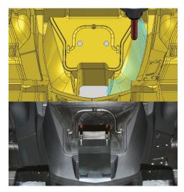
NX CAM tool path and machined part.
