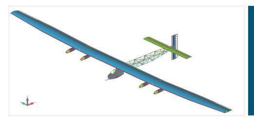
Femap with NX Nastran is being used to optimize and verify the structure of first plane to circumnavigate the earth using solar power alone
