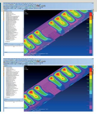
As an example of how the analysts use both imported geometry and the modeling tools within Femap, Piller describes some work done on the plane's wing structure. The analysts initially used the CAD geometry of the wing's outer surfaces to create a simple analysis model in order to look at load paths. Later, using Femap, they added 3D solid elements representing the Kevlar<sup>®</sup> aramid paper honeycomb core for more detailed analyses such as local and global buckling.
