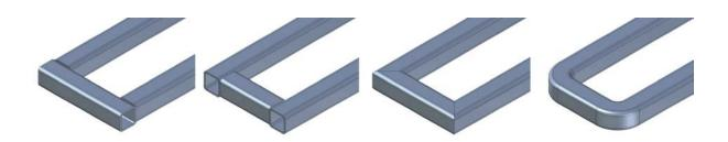
member will have material removed to suit). A butt2 condition is the opposite, with the shortest member being trimmed against. You can mix and match frame component sizes and shapes and their end condition treatments; any combination is possible.
