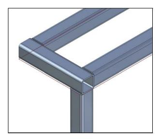
You can also select frame components and use standard SmartStep methodology to click back through any of the creation steps to edit a frame that you have already created. In this way, you can add or remove path segments, select new frame cross-section types or sizes, or change end treatments globally (for the whole frame) or locally (for a single vertex). After making edits, the frame will immediately be recomputed to show the changes.
