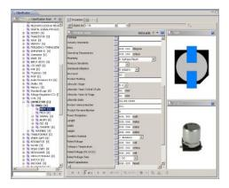
After the parts data is imported into Teamcenter, all ECAD parts are automatically classified in targeted libraries or catalogs using classification and attribute mapping tables. By using the gateway for ECAD part library to import the libraries, engineers can use the classification capabilities in Teamcenter to quickly identify and select the "right" part, while also ensuring the use of existing "preferred" parts.
