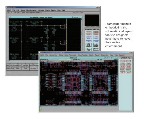
ECAD viewer technology. These capabilities allow users to investigate and identify potential issues early in the design process, thereby eliminating unnecessary scrap and rework.
