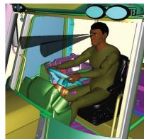
**4. Experience virtual reality** Jack provides interface drivers to a wide range of motion capture hardware devices, including real-time, whole body trackers and data gloves. This capability enables you to experience your design first hand, to quickly identify human factors issues, and to discover alternative processes and designs that will improve your product.
