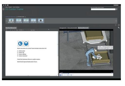
The EWI solution provides clear information about which parts and tools to use, reference documents, manufacturing instructions and more. It can also be integrated with the manufacturing execution system (MES) interface, enabling shop floor workers to access work instruction directly from the MES. The web interface is intuitive, making it easy to learn and use EWI with minimal training.
