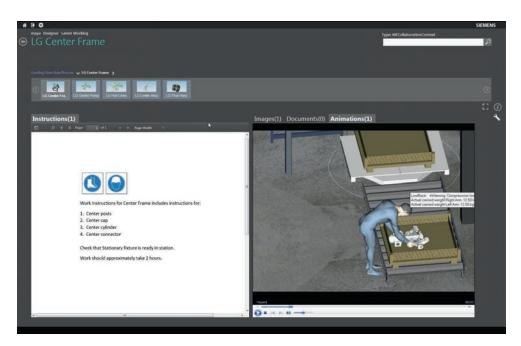
The EWI solution provides clear information about which parts and tools to use, reference documents, manufacturing instructions and more. It can also be integrated with the manufacturing execution system (MES) interface, enabling shop floor workers to access work instruction directly from the MES. The web interface is intuitive, making it easy to learn and use EWI with minimal training.
