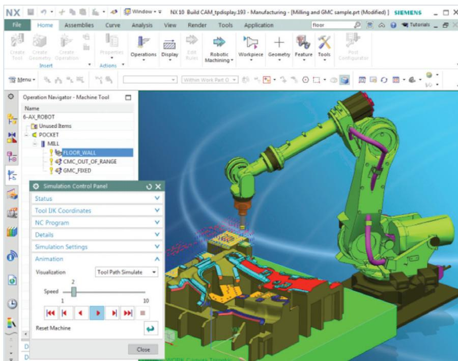
With NX CAM Robotics Programming, you can easily create cutting, trimming or grinding motions and simulate the robot as it performs the role of the machine tool.
