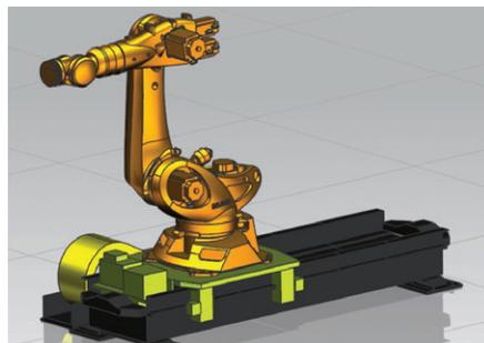
rail to increase its work envelope even further with this additional axis. NX CAM Robotics allows the robot to move along the rail to a specific position from where it can reach the entire toolpath, or continuously move back and forth to ensure all locations can be reached.
