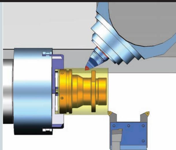
NX provides the manufacturing engineer with a single platform for part preparation, tooling and fixture design, CAM and CMM programming
