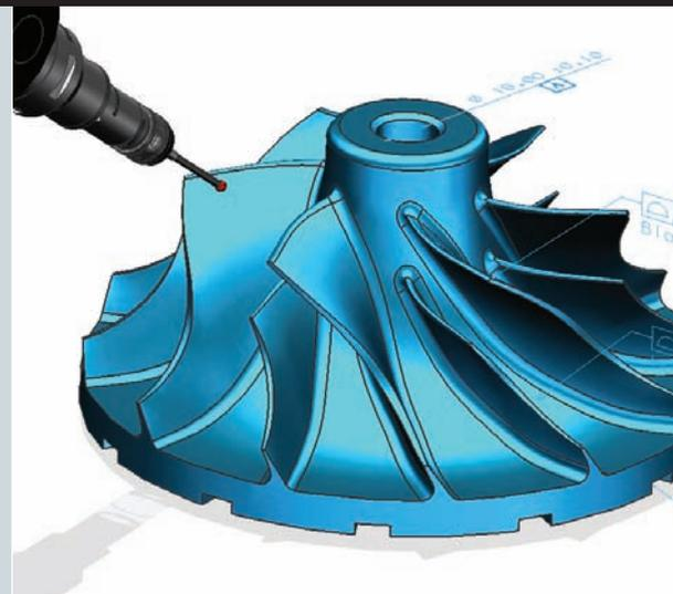
NX uses design requirements to automate the programming of CMMs directly from the model-based measurement and tolerance annotation (PMD)
