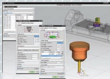
**3** NX CAM provides the environment in which to create, optimise and output the NC code required to drive all manner of machine tools and cutters
