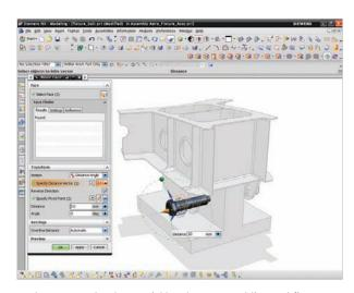
Synchronous technology quickly adapts assemblies and fixtures to accommodate new parts.
