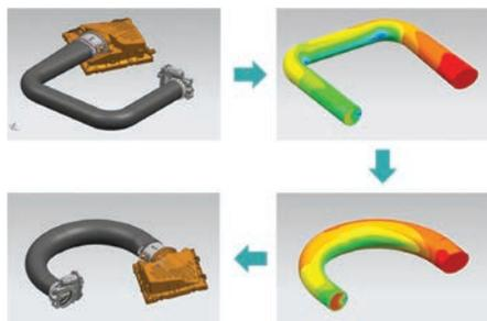
Drive design through simulation-based geometry optimization.
