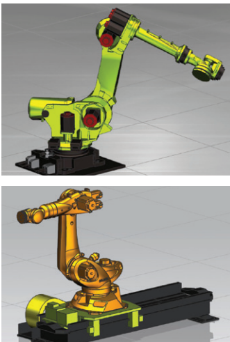
Six- and seven-axis robotic configurations can be defined and used in NX, including robots on rails and work positioners.
